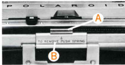
2. To remove it, push spring (A) and lift hinge (B). To replace, slide hinge down over spring.
